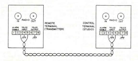
FIGURE 2 - I 2-WIRE TELCO COMMUNICATIONS
