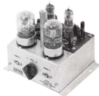
Open and closed views of the new ovenless, low drift crystal oscillator — first IPA unit.
