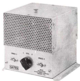
Open and closed views of the new ovenless, low drift crystal oscillator — first IPA unit.
