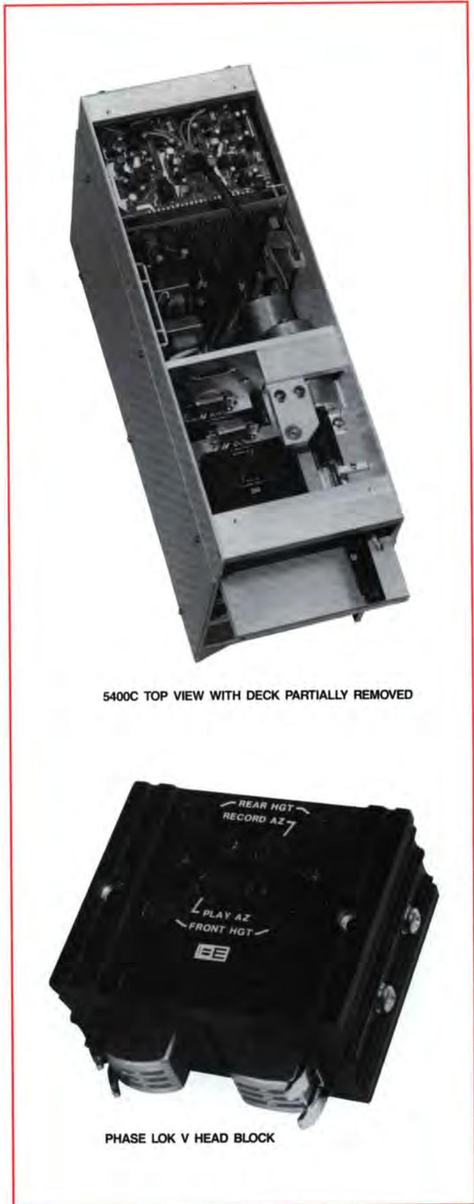
5400C TOP VIEW WITH DECK PARTIALLY REMOVED
