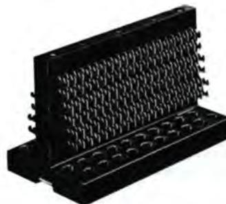
The ADC 20-Pin Terminal Blocks are molded of durable, black, thermoset plastic per Military specifications MIL-F-14F. Terminals are brass with a tin alloy plating for lasting solderability. The PJ-101 series blocks have terminals graduated in length for ease of wiring. All Terminal Blocks are numbered along the top row for easy terminal identification.
