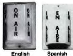
The STUDIO WARNING LIGHT is designed to mount to a flush wall or ceiling surface in a vertical or horizontal plane. The silkscreened globe housing fastens to a steel mounting plate. Ideally suited for control rooms, studios and above restricted entrances to live studios. Supplied complete with 25 watt red bulb and "Attention-Getter" flasher. Rated at 120V, 100 watts; UL approved. Available in Spanish, Portuguese or other languages. Special lettering also available.
