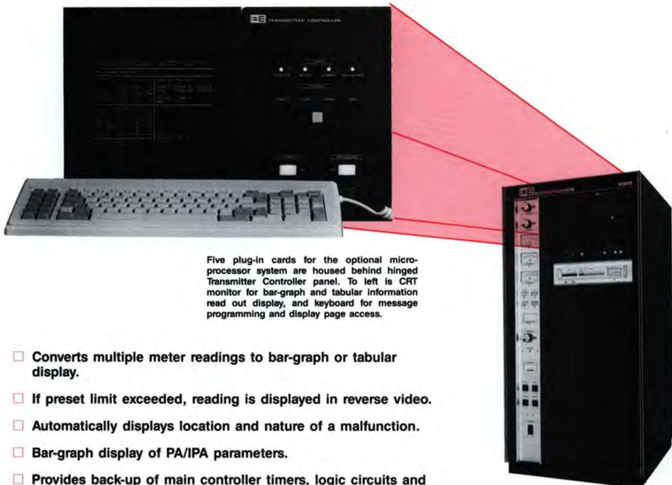
Five plug-in cards for the optional microprocessor system are housed behind hinged Transmitter Controller panel. To left is CRT monitor for bar-graph and tabular information read out display, and keyboard for message programming and display page access.
