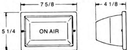
The STUDIO WARNING LIGHT is designed to mount to a flush wall or ceiling surface in a vertical or horizontal plane. The silkscreened globe housing fastens to a steel mounting plate. Ideally suited for control rooms, studios and above restricted entrances to live studios. Supplied complete with 25 watt red bulb and "Attention-Getter" flasher. Rated at 120V, 100 watts; UL approved. Available in Spanish, Portuguese or other languages. Special lettering also available.
