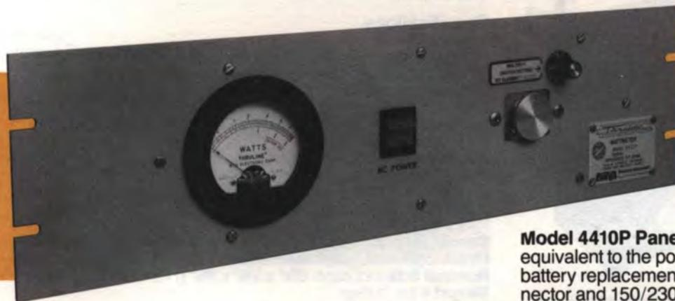
**Model 4410P Panel-Mounted Wattmeter** is electrically equivalent to the portable model 4411. It has a side door for battery replacement, a Universal Instrument-type AC connector and 150/230V rear selector switch, and fits into 5 $\frac{1}{4}$ " space of standard 19" racks. RF Quick-Change Connectors can be changed without dismounting the 4410P from its rack.
