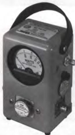
This THRULINE® Wattmeter is similar to model 4431 above, except for a fixed RF tap. RF coupling is approximately -53dB from 512MHz down to 10MHz, and decreases to
