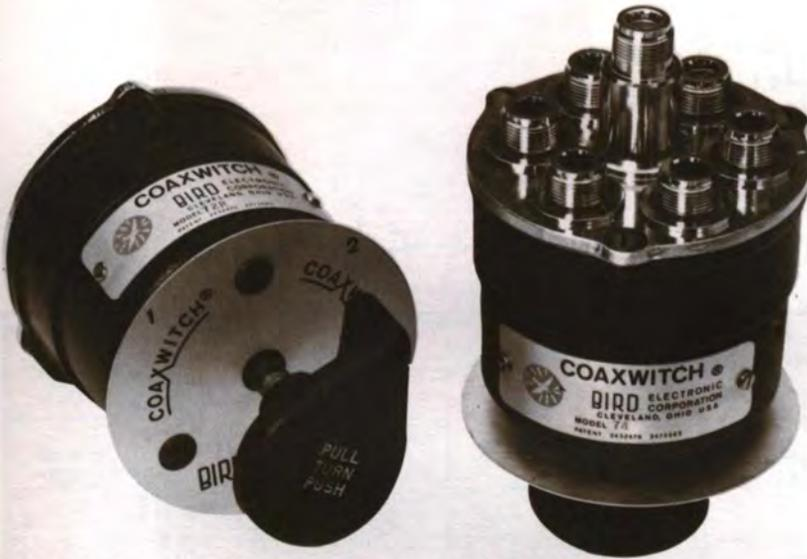
**Description:** BIRD COAXWITCH Coaxial Selector Switches employ a unique, rugged and reliable design which permits positive contact, low insertion VSWR, and negligible cross talk between channels. The switching mechanism is 4½" of RG-87/U Teflon cable which is pulled away from the mating Male N connectors and rotated to the desired switch position. 75 ohm versions of all models shown available on special order.
