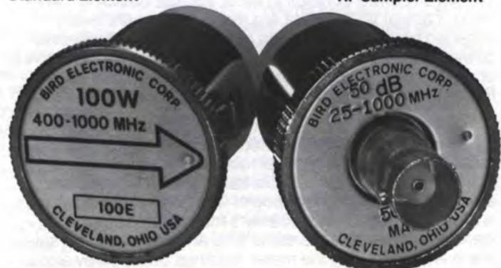
*Coupler Elements: For RF signal observation on a scope, for spectrum analysis or for frequency counting and control, use Model 4274-025 wide range RF Sampler Element. This non-directional coupler delivers an unrectified signal at about -50dB ±2dB from 25-1000MHz tapering down to -66dB at 2MHz. Main line power should not exceed 500W.*
