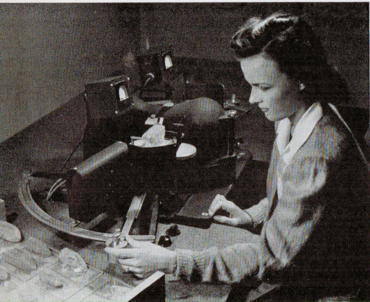
Philips X-ray inspection, above, assures correct wafer cutting in relation to crystal ZZ' angle. In room below, the rough crystal blocks are cut into wafers. Close view, right, shows how high-speed, diamond-edged circular saw cuts through hard quartz with ease, slicing off wafers which are then separated for further processing and frequent inspection.
