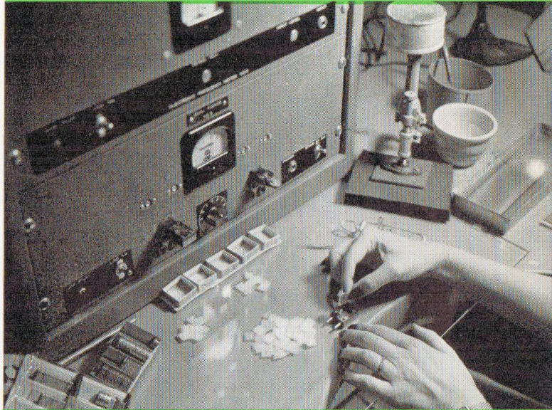
Another view , below, of the final finishing, assembling and frequency tests operations which assure extra precision quality in Monitor crystals.
