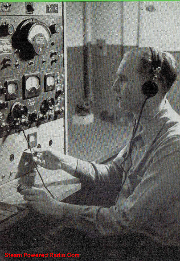
All Monitor Crystals are subjected to activity and frequency tests under extreme temperatures ranging from as low as minus 50° Centigrade to as high as 90° Centigrade in the special equipment shown above. Below, The Army Signal Corps' civilian resident inspector subjects all Monitor crystals to a final, rigid inspection before acceptance for delivery.
