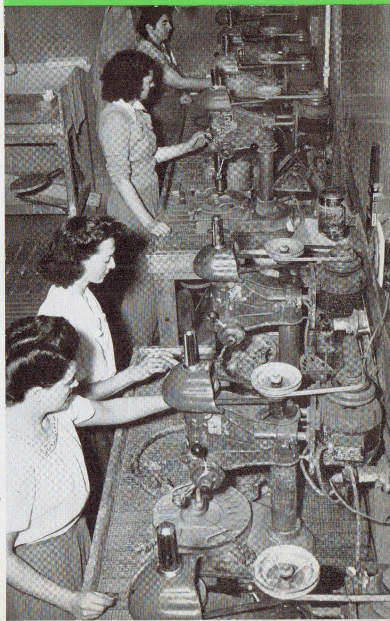
Electric micrometer checks thicknesses to .0001". Below, blanks are "lapped" or ground to desired thicknesses in these machines.
