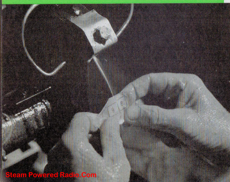
Wafers are diced into "blanks," above, on high-speed circular saws. Close view, below, shows how wafers have been stamped as a guide in cutting so that the greatest number of blanks are obtained from each wafer. Two sides of each blank are "squared," below, to fit the vise-like "jig" holder used in truing the blanks to perfect squares.
