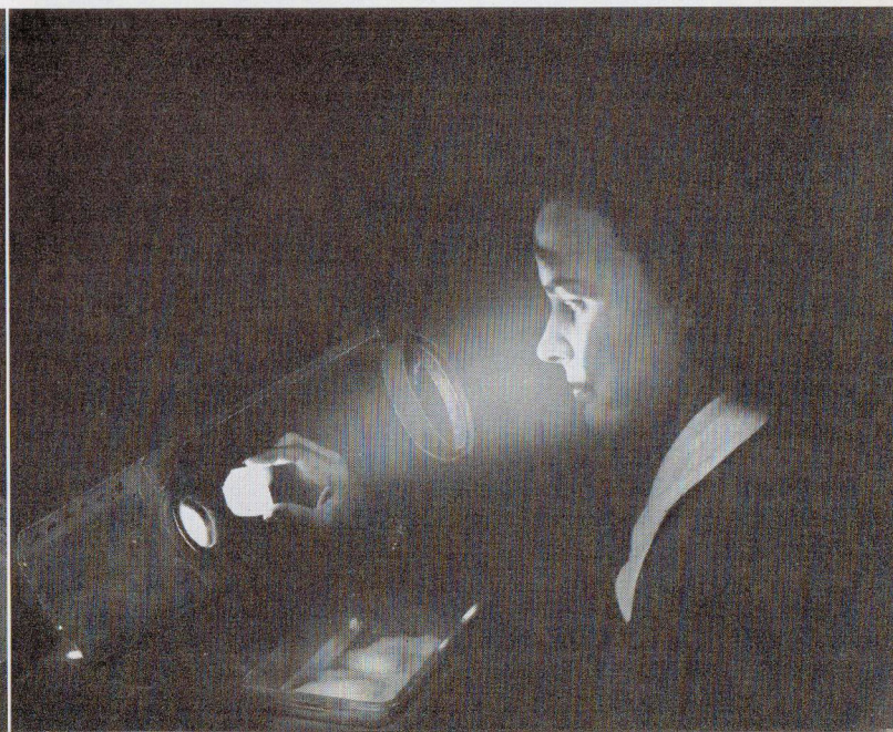
POLARISCOPE REVEALS UNUSABLE "TWINNED" AREAS
