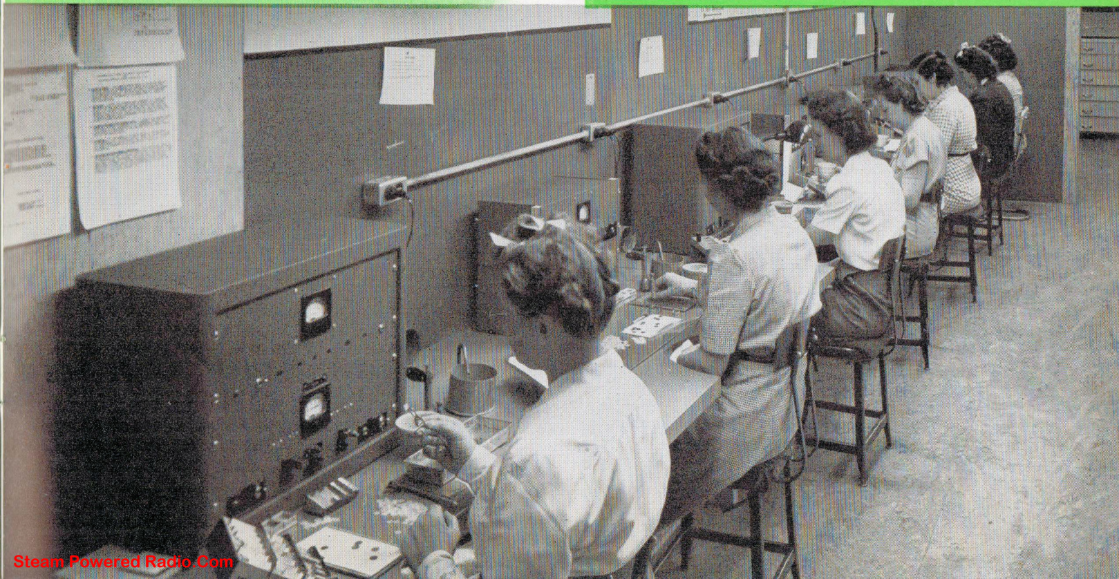
Another view , below, of the final finishing, assembling and frequency tests operations which assure extra precision quality in Monitor crystals.
