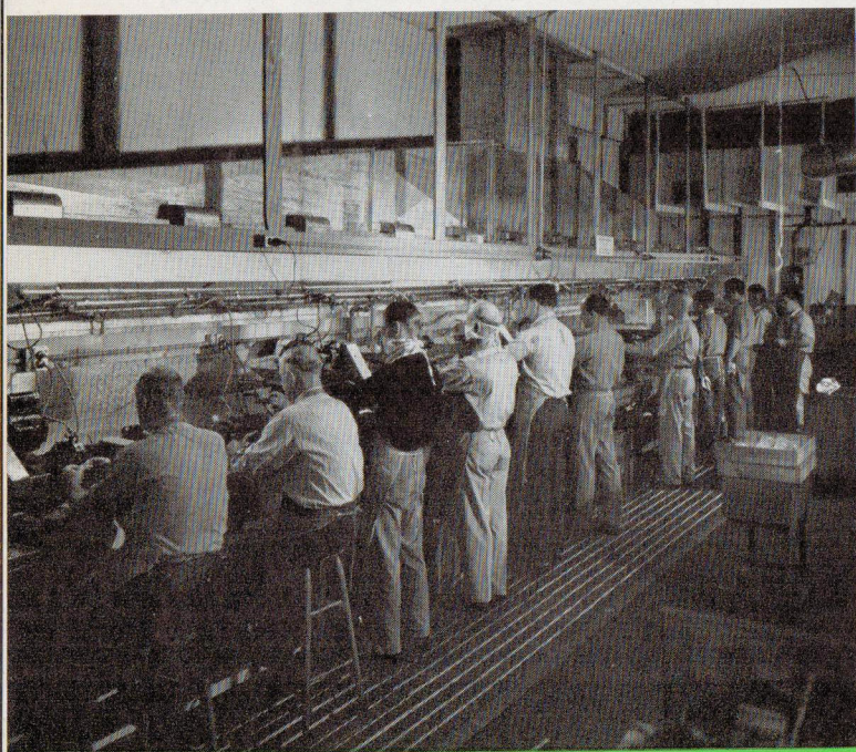
Wafers are diced into "blanks," above, on high-speed circular saws. Close view, below, shows how wafers have been stamped as a guide in cutting so that the greatest number of blanks are obtained from each wafer. Two sides of each blank are "squared," below, to fit the vise-like "jig" holder used in truing the blanks to perfect squares.
