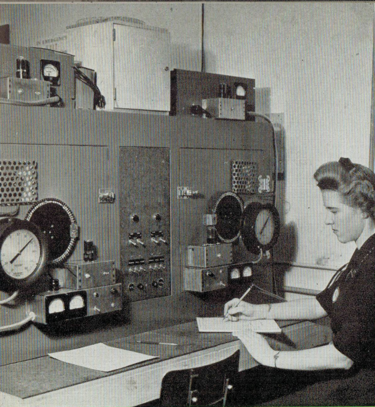
All Monitor Crystals are subjected to activity and frequency tests under extreme temperatures ranging from as low as minus 50° Centigrade to as high as 90° Centigrade in the special equipment shown above. Below, The Army Signal Corps' civilian resident inspector subjects all Monitor crystals to a final, rigid inspection before acceptance for delivery.
