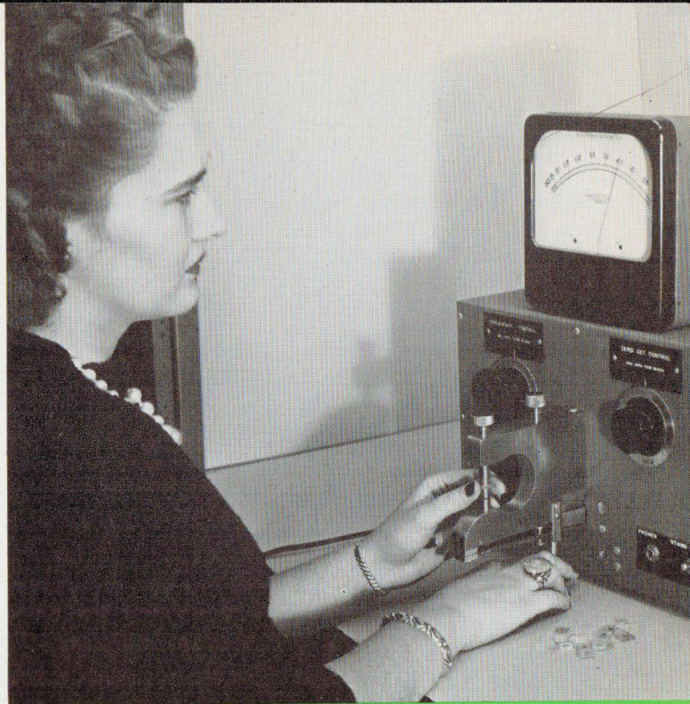
Electric micrometer checks thicknesses to .0001". Below, blanks are "lapped" or ground to desired thicknesses in these machines.
