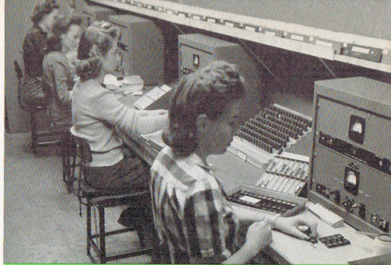
Final assembly , where finished crystals are checked for frequency and activity and mounted in crystal holder as shown in close view below.
