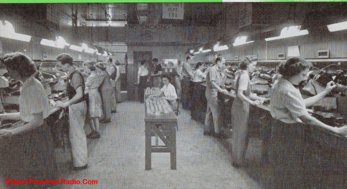
Philips X-ray inspection, above, assures correct wafer cutting in relation to crystal ZZ' angle. In room below, the rough crystal blocks are cut into wafers. Close view, right, shows how high-speed, diamond-edged circular saw cuts through hard quartz with ease, slicing off wafers which are then separated for further processing and frequent inspection.
