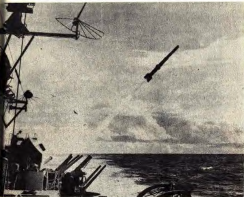
U. S. Navy Rat being launched from a destroyer. At the end of its flight path, two parachutes lower the torpedo into the water.
