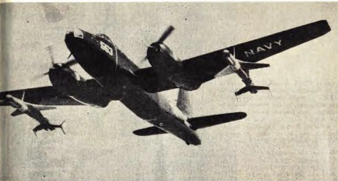
U. S. Navy Petrel missiles mounted beneath wings of Lockheed P2V6-B.
