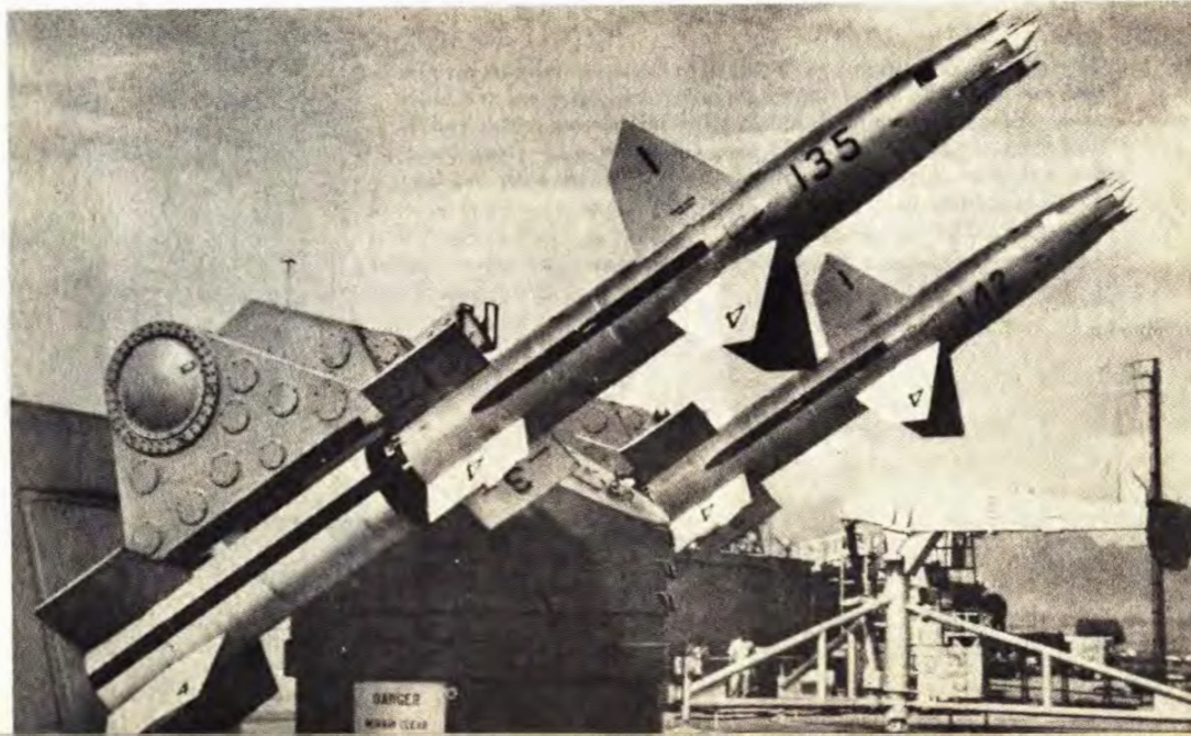
U. S. Navy Talos missiles on the Navy's "U.S.S. Desert Ship" at White Sands Proving Ground. Installation is similar to that aboard ship.
