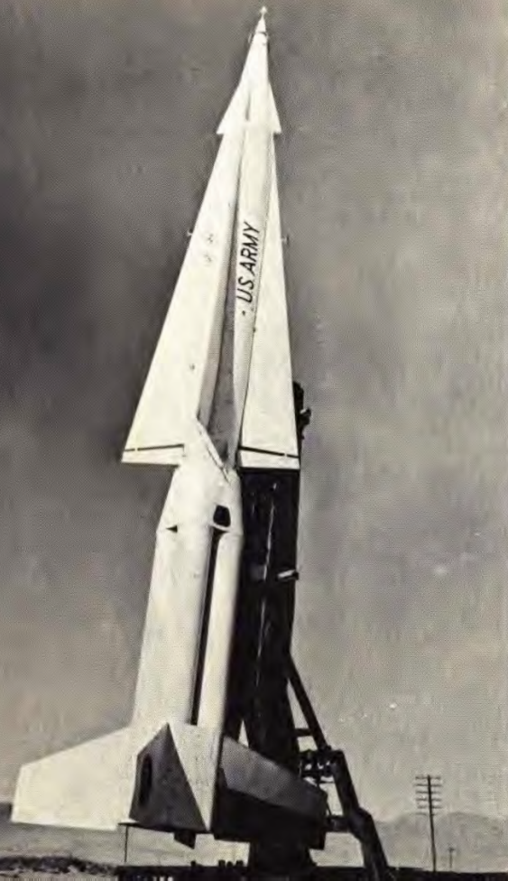
U. S. Army Nike-Hercules in launching position at White Sands Proving Ground. Tubes in bottom half of missile are booster rockets.
