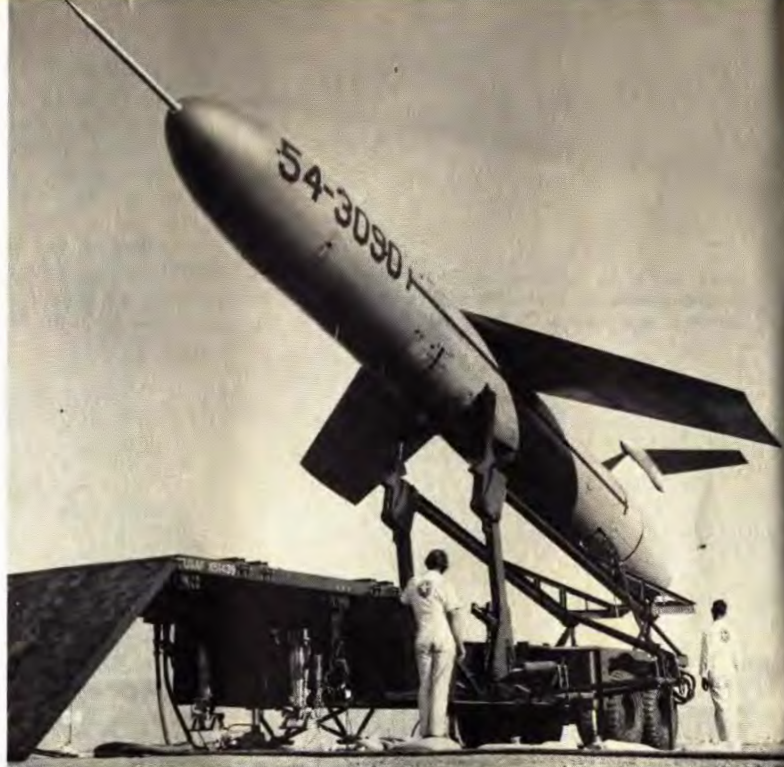
USAF Matador being readied for test flight from its portable transporter-launcher. Solid-fuel booster has not yet been mounted beneath the tail of the missile.
