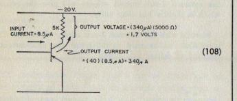
Therefore, the voltage gain of the amplifier is:
