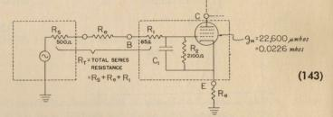
which means that a resistance equal to  $R_e$  must now be included in  $R_T$ , the total series resistance. If the value of  $R_e$  is, for example, 300 ohms, the new bandwidth is:
