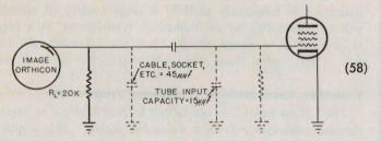
In this circuit a total of 60  $\mu\mu$ f of stray capacity shunts R<sub>L</sub>, the 20K load resistor. If the stray capacitance were less, a larger load resistor could be used. The signal voltage available at the grid of the tube would then be greater, in direct proportion to the size of the load resistor. As the circuit now stands, however, 20K is about the largest practical value of load resistor.
