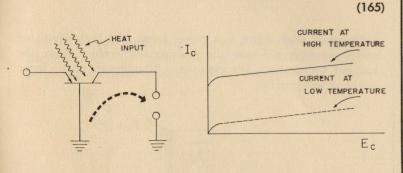
The increase is very rapid; the current doubles about every 9 C. However, even at the highest operating temperatures, this relatively small current does not often cause trouble as long as the base is grounded.
