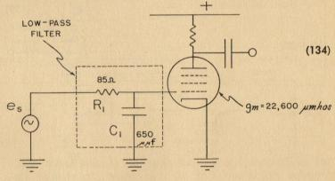
The 70 percent response point of the low-pass filter is at a frequency
