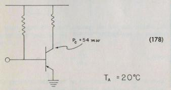
then a thermal resistance of 0.5 C/mw tells us that the junction temperature is higher than the ambient by
