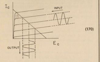
If the temperature is raised, however, the curves shift upward, and the amplifier begins to clip:
