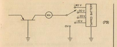
and the  $E_c$  vs  $I_c$  curves were determined; first for zero emitter current:
