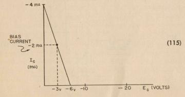
The actual CE characteristics have not been drawn on the foregoing graph purposely to show that the transistor characteristics have nothing to do with the approximate determination of the operating point. However, these characteristics must be included in order to calculate gain:
