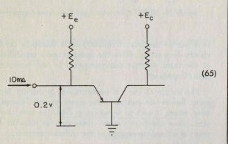
The transistor can be given a collector load which will give the same signal voltage gain as the 10-to-1 step-up transformer:
