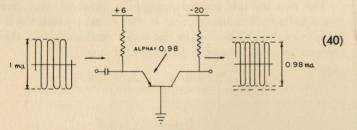
The voltage gain (the ratio of output to input voltages) can be calculated from the output and input impedances. The output impedance, in this case, is known to be a 5000-ohm resistor, but the input impedance was stated vaguely to be "less than 50 ohms." Fortunately, there is a simple way to calculate the input impedance (emitter resistance). It is given by the formula<sup>5</sup>:
