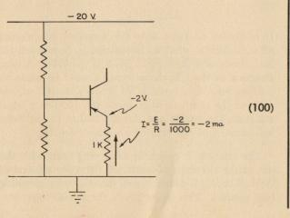
Assuming that  $\alpha = 1$  (instead of 0.98) for this approximation, the current flowing from the collector is also -2 ma, and the potential at the collector is therefore -10 volts:
