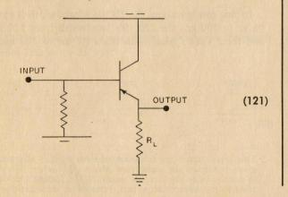
a transistor with a beta of 49 will give a current gain of 50:
