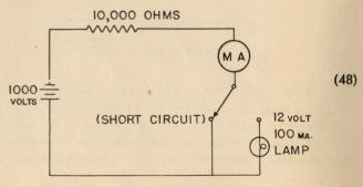
Note that a 1000-volt battery supplies current to a lamp when the switch is thrown.
