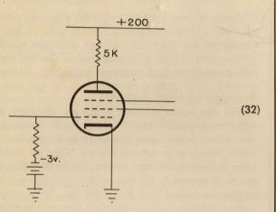
will have a load line connecting the 200-volt point and the 40ma point, (the 40-ma point is obtained by dividing 200 volts by 5,000 ohms):
