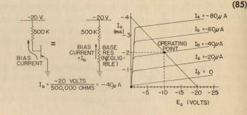
This common-emitter amplifier therefore operates with a bias current of 40  $\mu$ A, a collector current of -2 ma, and a collector voltage of -10 volts:
