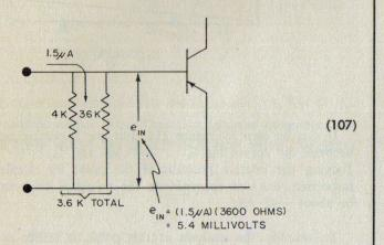
At the same time, 8.5  $\mu$ A is being amplified by the transistor so that (8.5)  $\times$  (40) = 340  $\mu$ A appears as a current swing in the load resistor, and an output of 1.7 volts appears across the load resistor:
