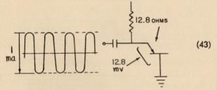
Almost all of the 1-ma signal current (98 percent of it) flows in the 5000-ohm load resistor, producing a 5-volt drop across it:
