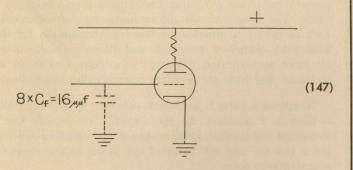
In transistors, a similar effect takes place. If the load resistor is large enough to give a useful gain, then a feedback capacity  $C_f$  which appears in this manner;
