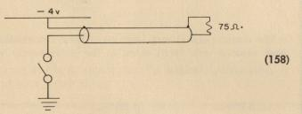
Every time the switch is closed and then opened, a 4-volt pulse appears across the 75-ohm resistor. If the switch is replaced by a transistor which is driven into saturation by an input pulse,
