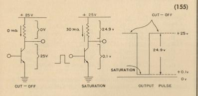
In this case, the transistor dissipates (during the pulse) only
