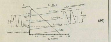
Since the output current is only 1.6 ma (instead of 2 ma, as it was for the short-circuit load) (88), the current gain of this amplifier is:
