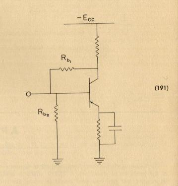
The common-base amplifier with current bias exhibits the best obtainable single-stage temperature independence. However, it lacks the gain capabilities of the common-emitter configuration. Some circuits can be arranged to make use of the good features of both the CE and CB configurations. This is accomplished by making the amplifier a CE configuration for signal currents:
