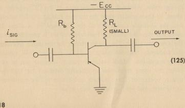
will provide a bandwidth of about 16 kc for a 2N104; about 120 kc for a 2N219, and about 1700 kc for a 2N384:
