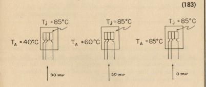
or, to put it another way, if this transistor has a 50-mw power input (for example), the ambient temperature must not rise above 60 C, or the junction temperature will exceed 85 C. Moreover, at an ambient temperature of 85 C, the transistor cannot be operated at all, since it cannot tolerate any power input.
