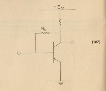
In this arrangement, any increase in collector current causes the voltage at the collector to decrease, thereby decreasing the bias current flowing through  $R_b$  into the base. When base current decreases, the collector current also decreases, thereby tending to restore the original operating condition.
