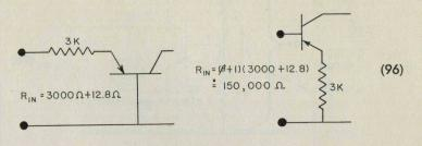
This external impedance, however, behaves like an unbypassed cathode resistor in a tube circuit—it gives higher input impedance (and greater stability as well) at the expense of gain.
