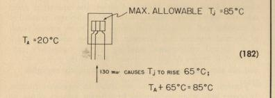
At this ambient temperature, 130 mw is the maximum allowable power input. At higher ambient temperatures, the maximum allowable power input is less than 130 mw:
