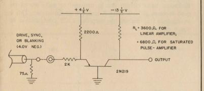
*Remarks:* The 2N219 shown here can be replaced by almost any PNP transistor, although audio-type transistors (such as the 2N109) will give poorer pulse performance. To use an NPN transistor, change the  $-13\frac{1}{2}$  volts to  $+13\frac{1}{2}$  yolts, and the  $+4\frac{1}{2}$  volts to  $-4\frac{1}{2}$  volts. For saturated operation with an NPN transistor, omit the 2200-ohm resistor and the  $4\frac{1}{2}$ -volt bias supply.
