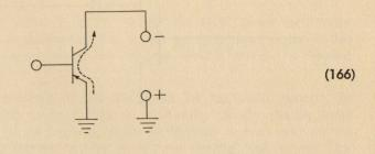
and in so doing, becomes amplified by the current-amplifying mechanism of the transistor. Consequently, the reverse current for the CE configuration is beta times greater than the reverse current for the CB configuration. With this larger current being doubled for every 9 C temperature rise, the high-temperature reverse current becomes a factor deserving serious consideration.
