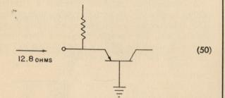
it must be fed from a source of even *lower* impedance in order to be conveniently classed as a voltage amplifier:
