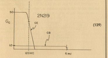
In the common-base case, the frequency at which the current gain is down 70 percent (6 mc for the 2N219) is called the *alpha cut-off frequency*,  $f_a$ . It is the frequency most commonly given in transistor data sheets, and is related to  $f_\beta$  by the expression:
