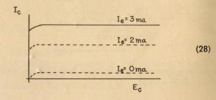
By selecting several different values of emitter current and showing a curve for each one, we can generate an entire family of curves:
