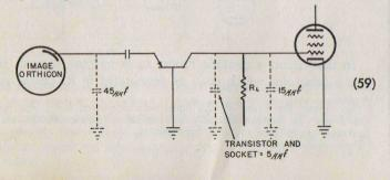
Note that only  $15 + 5 = 20 \ \mu\mu$ f appears across the load resistor. Since this is only 1/3 of the 60  $\mu\mu$ f of the first circuit,  $R_L$  can be 3 times as big, or 60K. The result is an *effective* gain of three.
