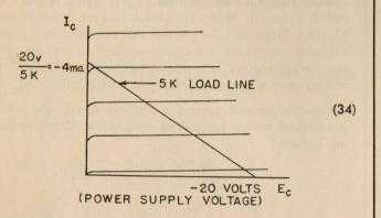
Just as for vacuum tubes, the operating point of the transistor amplifier must lie somewhere on its load line. For the pentode, the operating point lies at the intersection of the load line and the curve representing the particular bias chosen by the design engineer:
