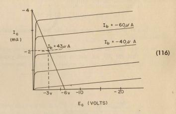
It can be seen in Figure 116 that the operating point lies between the curves for  $I_b = -40 \ \mu A$  and  $I_b = -60 \ \mu A$ . Judging the relative position of the point by simple visual inspection, one can approximate the no-signal base-current to be about  $-43 \ \mu A$ .
