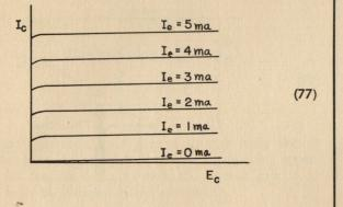
thereby generating the  $E_e$  vs  $I_e$  curves for the common-base configuration. With these curves the operation of a CB amplifier was analyzed.
