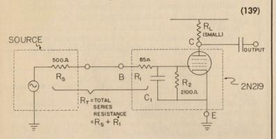
In this case, it can be shown that the original  $f_{\beta}$  bandwidth is improved by a factor of 4.6:
