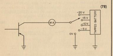
and its E<sub>c</sub> vs I<sub>c</sub> curves plotted; first for zero base current:
