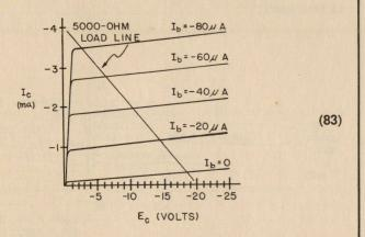
Just as for the common-base circuit, this amplifier's operating point must lie somewhere on its load line. For the commonbase amplifier, it was shown (38) that the operating point lies at the intersection of the load line and the particular biascurrent chosen:
