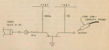
*Remarks*: The transistor used here should have an alpha cutoff frequency somewhat greater than the desired bandwidth. As shown, a low-capacity probe should be used to view the waveform. An NPN transistor may be used by reversing the polarity of the power supply voltages.
