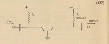
In this configuration, the 2N104's bandwidth is extended from 16 kc to 700 kc; the 2N219's bandwidth from 120 kc to 6 mc; and the 2N384's bandwidth from 1.7 mc to 102 mc:
