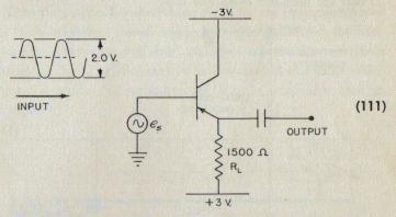
This amplifier is driven from a very-low-impedance source which approximates a true voltage source. This amplifier's voltage gain and its dc operating conditions will be determined by a construction on the common-*emitter* curves.
