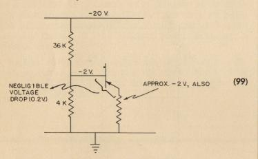
Therefore, the emitter is also at approximately -2 volts. Since the emitter resistor is 1,000 ohms, the current to cause this 2-volt drop must be -2 ma.
