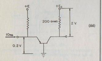
The signal current, however, at the output is not reduced proportionally, but instead is virtually the same as the input current:
