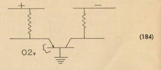
at higher temperatures has a smaller drop. This effect is of no consequence when the emitter is current-biased,
