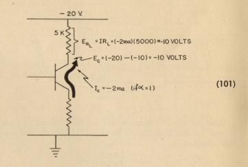
Since the emitter is at -2 volts, the voltage across the transistor is only -8 volts; therefore the power dissipation is:
