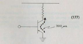
If the simple single-resistor biasing technique is used (to exaggerate, for this example, the effects of temperature), and the circuit is adjusted for 54 mw dissipation,
