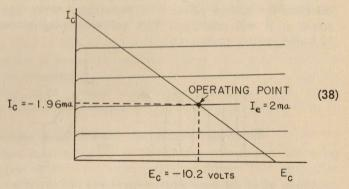
This transistor amplifier therefore operates with a bias current of 2 ma, a collector current of -1.96 ma, and a voltage at the collector of -10.2 volts:
