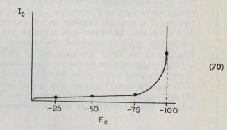
The voltage at which the curve breaks sharply upward is called the *breakdown voltage*. In this region, a transistor does not behave normally. To insure proper transistor action, the operating point must be well removed from the breakdown region.
