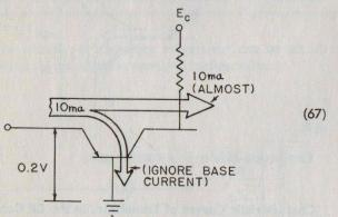
Therefore, the signal power at the output is ten times greater than at the input:
