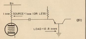
This is not always practical. Transformers may be used to obtain such low impedances in narrow-band or tuned amplifiers,
