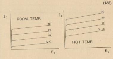
This displacement can seriously disturb the functioning of an amplifier. Consider the effect that elevated temperatures would have on this simple CE amplifier:
