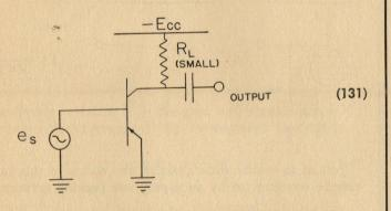
For the 2N219, this circuit arrangement extends the frequency response from 120 kc to 2.9 mc:
