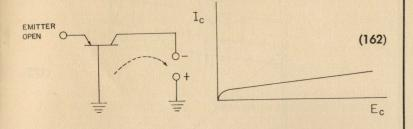
This current has two components. The first component results from simple resistive leakage paths,
