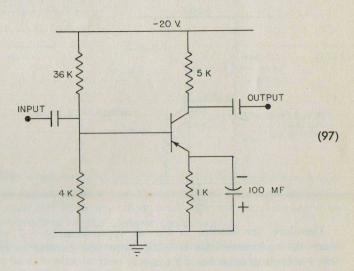
It is desired to know how this amplifier is operating; that is, what its bias is, what its dissipation is, how much collector current flows, and how much gain it provides. Although a construction of the CE characteristics could be made to yield this information, it is possible to make a fairly accurate analysis without the characteristics, since the 1000-ohm emitter resistor stabilizes the circuit and thereby makes its d-c behavior fairly independent of the transistor's characteristics.
