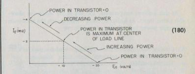
When the operating point is on the lower half of the load line, an increase in current causes an increase in power; this is thermal regeneration. When the operating point is on the *upper* half of the load line, an increase in current causes a *decrease* in power; this is *thermal degeneration*.
