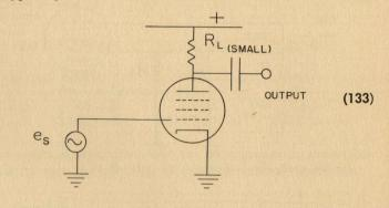
would have a bandwidth several times greater than the transistor bandwidth, but its gain would be only one-half to one-third as great. It would be possible to make a tube circuit which would behave almost like a 2N219, but to do so would require a pentode with a high transconductance—more than 22,000 umhos —and would also require the use of a low-pass filter in the grid circuit, to simulate the poor frequency response of the transistor:
