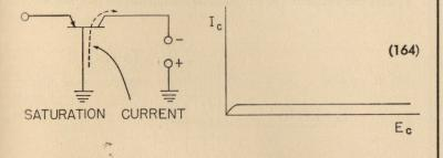
Although the saturation current is little affected by changes in collector voltage, it is extremely sensitive to changes in temperature. As junction temperature is increased, the saturation current increases:
