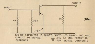
If a signal current of 10  $\mu$ A is supplied to this amplifier, part of it is lost in the 4K and 36K resistors. Only a portion of it goes into the base (represented here by a 650-ohm resistor):
