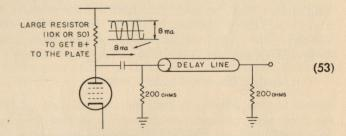
In this circuit a pentode drives an 8-ma peak-to-peak signal into a delay line which *must* be terminated in its characteristic
