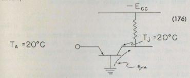
it will have a reverse current of  $\beta \times 6 \mu a = 300 \mu a$  in this circuit:
