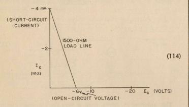
Actually, drawing a straight line between the two end points determined in the above manner is not entirely accurate because the current scale of the graph is  $I_c$ , whereas it is really  $I_e$  which flows through  $R_L$ . However, the error involved is small since  $I_c$  and  $I_e$  are nearly equal.
