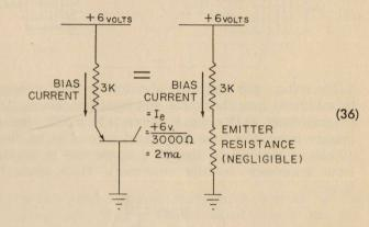
Since the emitter resistance is usually very small (less than 50 ohms), its resistance may be neglected in computing the bias current. The current is therefore:
