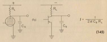
Just as in vacuum-tube practice, the effects of this capacity may be counteracted by an appropriate peaking network.
