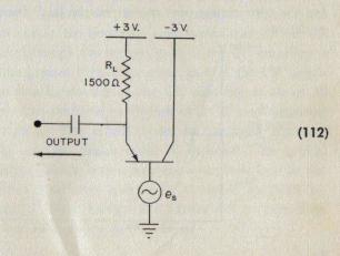
Remembering that e<sub>s</sub>, the signal source, is practically a short circuit to the bias currents, it can be seen that the biasing arrangement bears a strong resemblance to common-base biasing.
