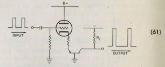
This circuit gives almost the same gain as the first circuit, and does not invert the signal.
