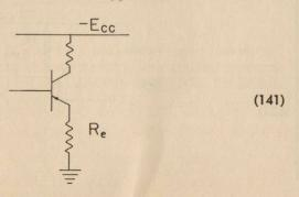
In this case, the beta cut-off frequency is extended by an even larger factor, as shown in this expression:
