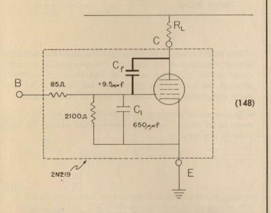
is magnified by a factor 1 + the gain, and appears across  $C_1$ . If the gain is 7, for example, then the magnified capacity is
