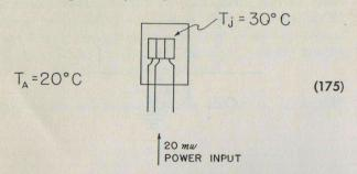
It is correct to deduce from these two cases that every 1 milliwatt of power input will cause a 0.5 C rise in junction temperature for this particular transistor. This characteristic of a transistor is called its *thermal resistance*, and would be listed in the data sheet of this particular transistor as having a value of  $0.5^{\circ}$ C/mw.
