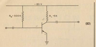
It is desired to know how this amplifier is operating—what the bias is, how much collector current flows, how much power is dissipated in the collector, and how much gain it will offer. All these facts may be ascertained by a simple construction on the common-emitter characteristics.
