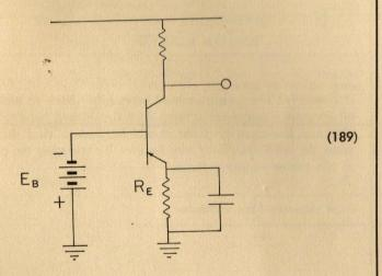
The emitter current (and therefore, the collector current) is determined principally by the "battery" voltage and the emitter resistor:
