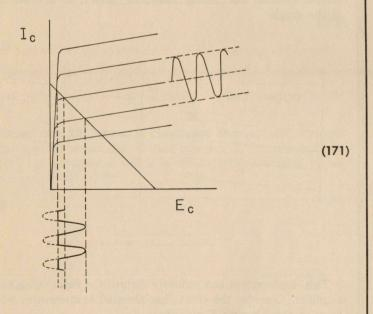
At a sufficiently high temperature, the signal is completely clipped,
