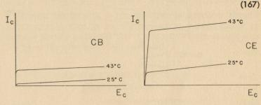
The family of curves is not distorted by the high-temperature reverse current, but merely displaced, intact, to another area of the graph:
