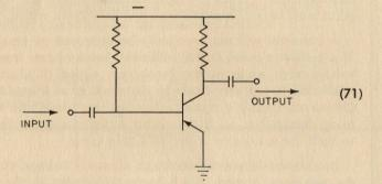
corresponds roughly to the grounded cathode configuration of a vacuum tube:
