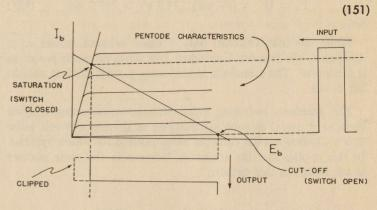
The output pulse is very large under these circumstances. Its peak value is very nearly equal to the power supply voltage:
