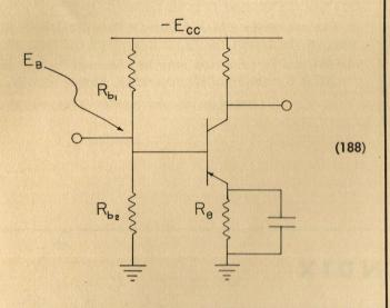
Here the fundamental requirement is that the bleeder current flowing through  $R_{b_1}$  and  $R_{b_2}$  be so much larger than the base current that changes in base current cannot influence the voltage at the midpoint of the  $R_{b_1}/R_{b_2}$  divider. Under this circumstance, the base voltage cannot change, and the circuit behaves like a biased-up common-base amplifier, insofar as the bias currents are concerned:
