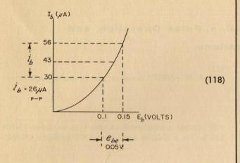
it can be seen that 0.05 volts of the input signal is lost in the base-to-emitter voltage drop. Therefore, in order to produce the assumed 2-volt output, the input voltage must swing 2.05 volts:
