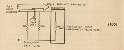
Since 15 percent of the input signal is lost before it ever gets into the base, the overall current gain of this amplifier is 15 percent lower than the gain of the simple amplifier already analyzed (90). (That amplifier lost a negligible amount of signal current in its 500,000-ohm biasing resistor.) Since that amplifier was shown to have a current gain of 40, this amplifier will have an overall current gain of:
