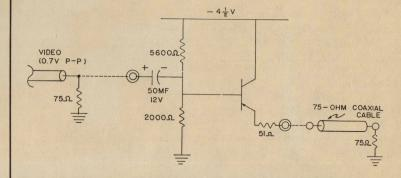
Remarks: This line-driver provides proper terminations for a 75-ohm line. It has a gain of one-half. Its bandwidth can be calculated from expression (142) in Part III.
