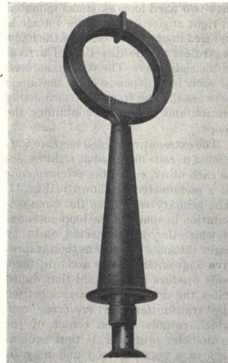
Typical Marine direction-finder loop. Notice the sturdy housing used to provide shielding and to protect the loop from the weather.
