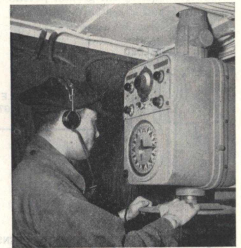
FIG. 15. This man is making a position fix with the R.M.C.A. AR-8709 direction finder.
