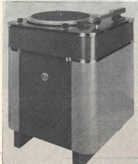
FIG. 18. An exterior view of the RCA type 70 transcription turntable used in broadcast programming. This unit operates at either 33-1/3 or 78.26 rpm, plays either vertically or laterally cut records and transcriptions, can accommodate records up to and including 16", and has 6 filter positions for altering the frequency response of records and transcriptions.
